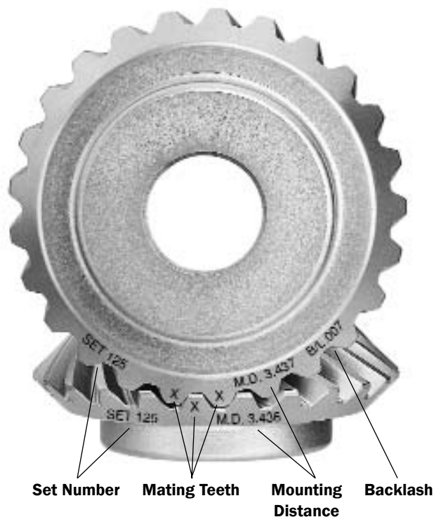
Fig. 29 - All Arrow Stock Gears are marked with the above assembly information.
