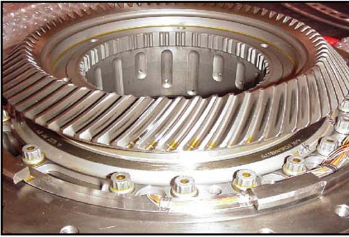
Fig. 8: Gear inspected after 75-hour run
